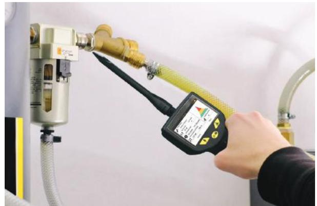
Leak detection with focus tube
