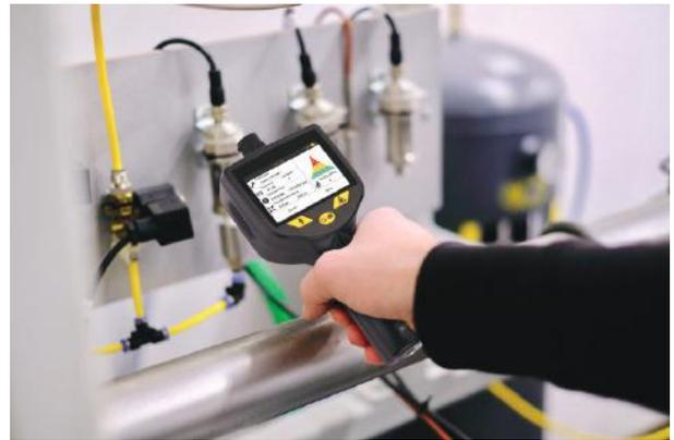
Ultrasonic Leak Detector S531
